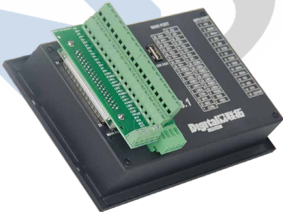
Figure 2-8 Main Port with wiring terminal
