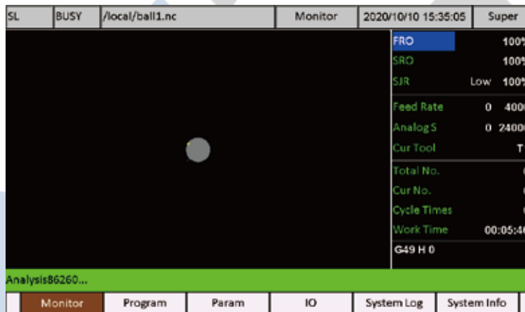
Figure 6-5 Preview the toolpath by Simulating a file
