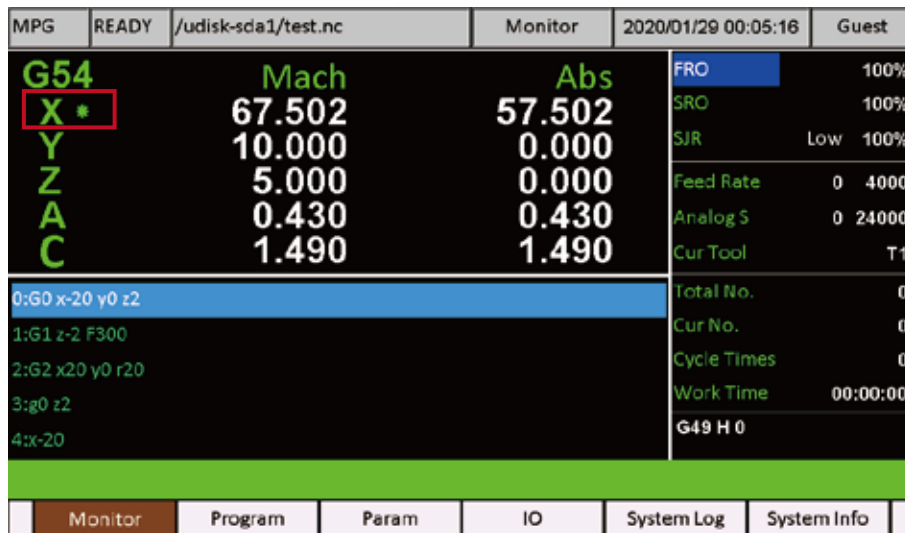
Figure 4-24 The MPG channel is on X axis
