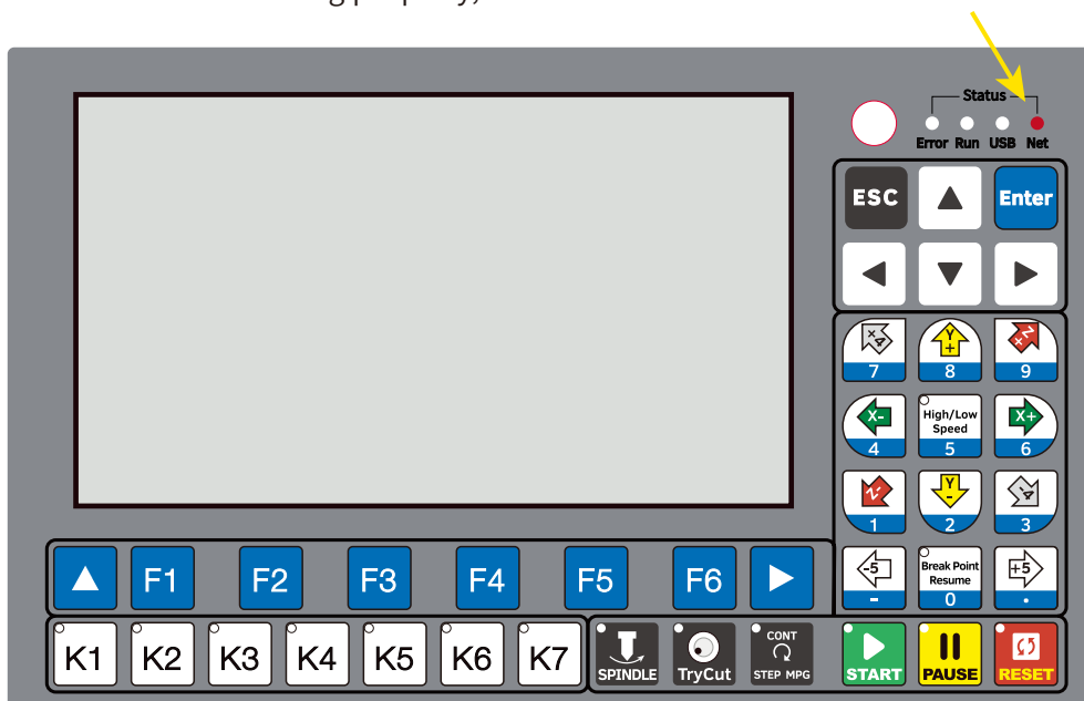
Figure 8-18 Network LED shows the status
