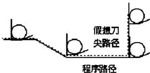
Figure 4-6 Tool path when programming with imaginary tool tip
