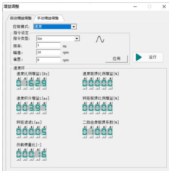
Figure 3-34 Speed-loop gain adjustment
